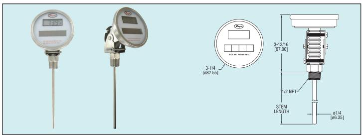
The Series DBT Digital Solar-Powered Bimetal Thermometer takes the guesswork out of temperature measurement. The 3-1/2 digit LED display is easy to read and provides resolution to 0.1°F. The adjustable angle can be mounted in virtually any position. The engineering units can be selected in the field by removing the back cover.
