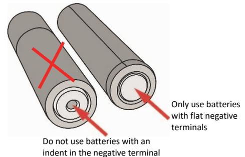
To install or replace the batteries:
