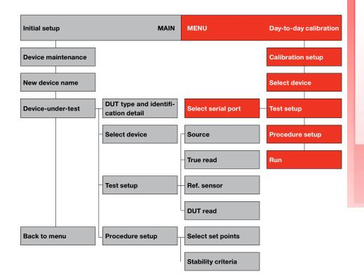
The unique "Icon bar" is key for easy set up of a calibration task. The "Icon bar" tells the current status of the calibration process, starting with selection of the sensor to be calibrated and ending with the performance of the calibration. The diagram shows the basic steps needed to set up a calibration.
