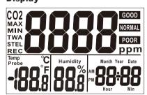
Upper LCD CO<sub>2</sub> reading Lower LCD Temp./Humidity/Real time display Carbon Dioxide reading MIN/MAX Minimum/Maximun readings TWA 8 hours Time Weighted Average STEL 15 mins short-term exposure limit GOOD CO2 value is in "GOOD" range NORMAL CO2 value is in "NORMAL" range P00R CO2 value is in "POOR" range Temp Temperature Probe temperature Probe Unit of relative humidity 0C/0F Celsius/Fahrenheit of temperature
