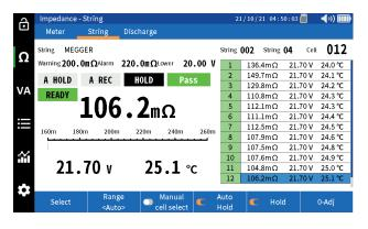
Discharge testing: measure cell impedance, voltage, and temperature
