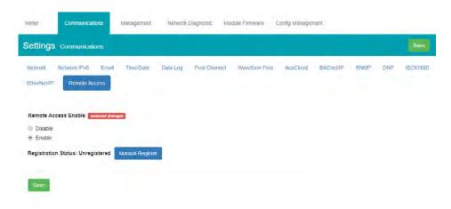
Users can click on the 'Manual Register' button to register the remote access. The following page will be displayed.
