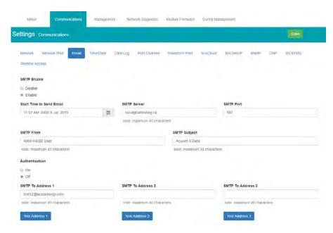
The content of the emails can either be time based triggered or event based triggered.
