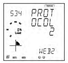
Once the protocol 2 setting of the Acuvim II meter is configured for WEB2, users can now view all necessary settings in the meters NET settings.
