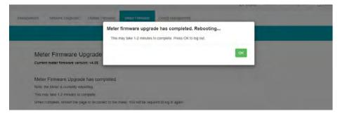
After the meter reboots, users will be able to log back into the web interface. When logged in click on the 'About' tab located on the top right corner of the web page to view the 'Device Information' page. From the Device Information page users can ensure that the meter was updated correctly to the right firmware version.
