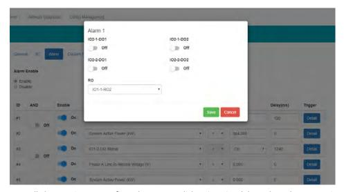
Once all alarm settings are configured, user must click on 'Save' and then reboot the communications module in order for the settings to be saved.
