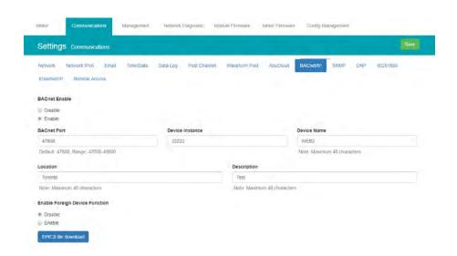
Under the "Enable Foreign Device Function", select 'Enable' to communicate with a BACnet device from another subnet.
