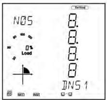
Press 'P' to get to "N06 DNS Secondary Server". Press 'V/A' to configure the DNS address.
