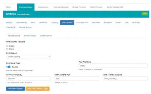
Select the Post Channel 2 tab to configure the settings for post to a second server.
