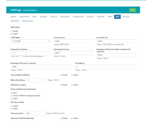
**DNP Enable:** Select 'Enable' to enable the function and to further configure the settings related to the DNP function.
