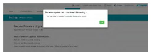
Login to the web interface of AXM-WEB2 after the reboot is complete, and go to the 'About' page to check if the module firmware version is updated.
