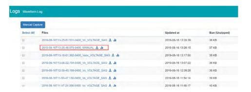
In the waveform log page, user also have the option to select and delete waveform files. Simply click on the check box next to the file to select it, alternatively users can click on the 'Select All' button. Once all files are selected click on delete to remove the files from the waveform log.
