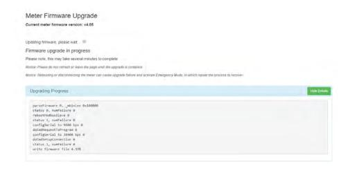
When the firmware update is complete, the module will reboot. The rebooting process will take 5-10 minutes to complete.
