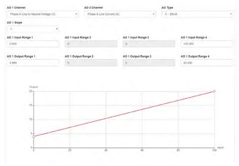
Similar to Analog Output channel 1, the second analog output channel can also be configured in the same manner from the web interface.
