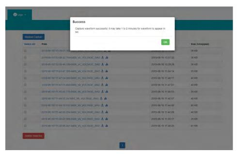
The file name for the manually captured waveform will include the timestamp the capture occurred and the reason will say 'MANUAL' at the end of the file.
