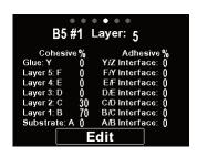
70% cohesive failure within layer 1; 30% cohesive within layer 2
