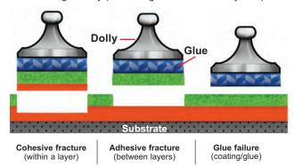
Glue failures typically occur when the glue is improperly mixed or the coated surface has not been adequately prepared (see pg.2).
