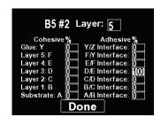
100% cohesive fracture at D/E coating interface (layer 3/layer 4)
