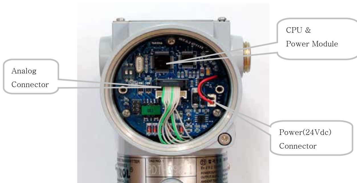
Figure 6.3 Structure of Electronics Module inner Transmitter
