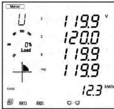
Figure 3-3 - Three-Phase Voltage Page
