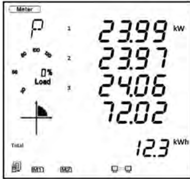
Figure 3-7 - Three-Phase Power Page
