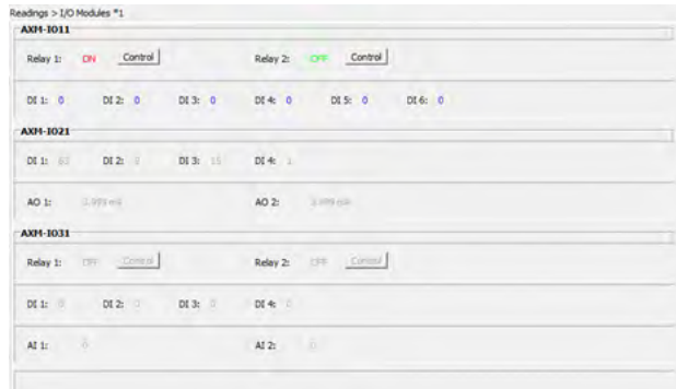
Figure 5-32 Relay Output Readings from Acuvim Software
