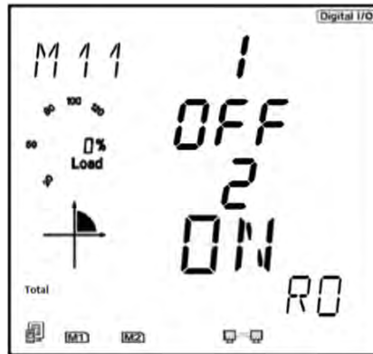
Figure 5-29 Relay Output Status Readings
