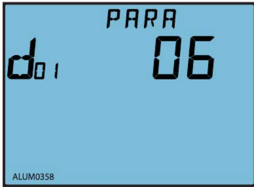
Fig.3-65 DO1 alarm output items setting
