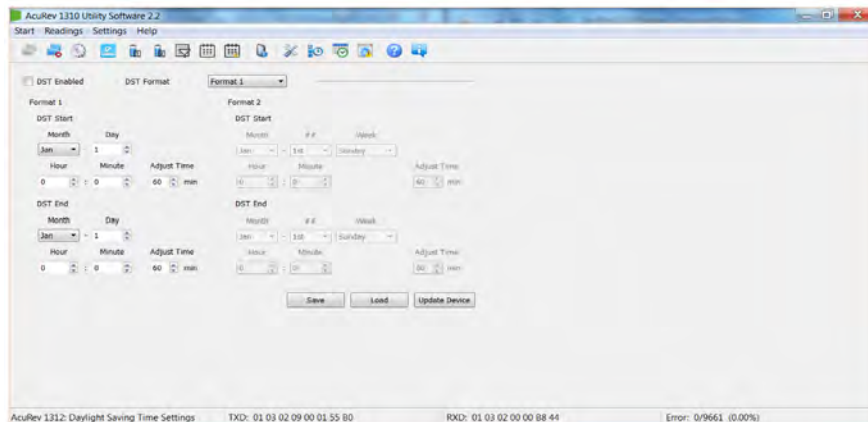
Figure 4-21 Daylight Saving Time Setting on Acurev 1310 Utility Software
