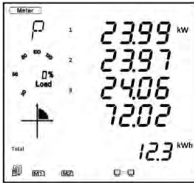
Figure 3-7 - Three-Phase Power Page
