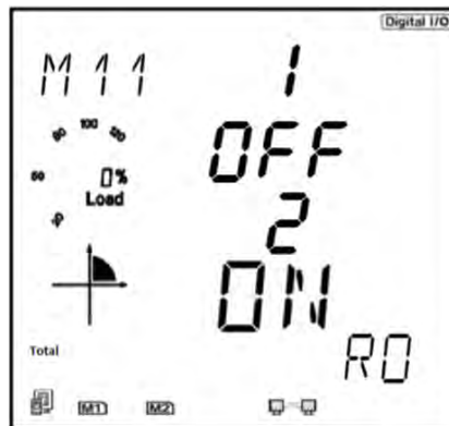
Figure 5-29 Relay Output Status Readings
