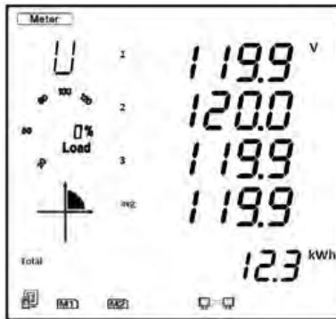
Figure 3-3 - Three-Phase Voltage Page
