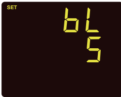
Fig 3-11 Backlight Brightness Setting
