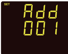
Fig 3-15 Communication Address Setup
