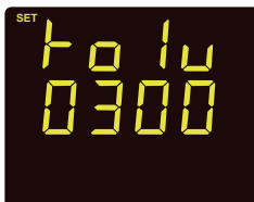
Fig 3-29 RO1 Alarm Threshold Range Setting
