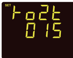
Fig 3-36 RO2 Alarm Delay Setting
