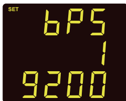
Fig 3-16 Baud Rate Setting
