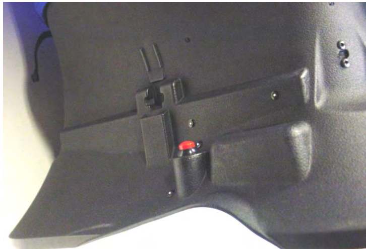
Figure 8 Red Hold Switch Location
