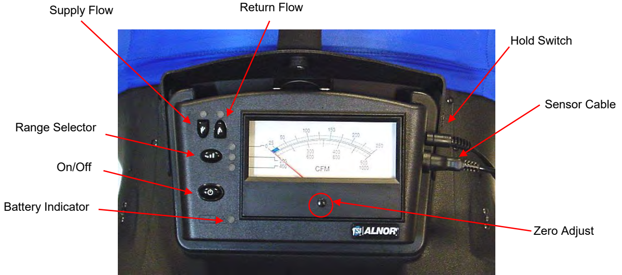
Figure 7 Analog Meter Components
