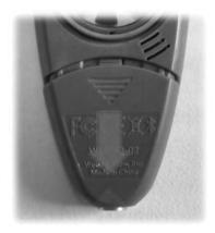
Step four: Replace battery with a CR2450 coin cell. The positive (+) faces away from the circuit board.
