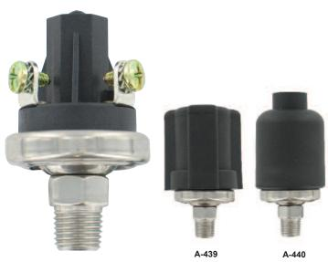
Series A6 Durable Pressure Switches have been specifically designed to stand up to extended duty applications. These switches are constructed with a polyimide film diaphragm and are compatible with a variety of fluids. For ease of installation, the switches come with a 1/4" male NPT process connection and can be mounted in any orientation. The Series A6 pressure switches are compact and have great setpoint integrity, and feature simple, easy set-point field adjustment.
