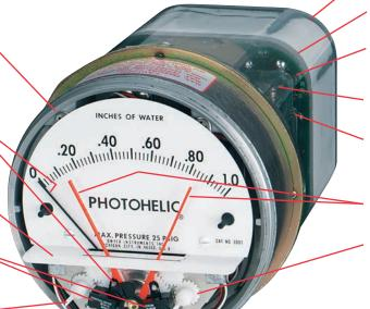
Plastic enclosure protects electronic components and electrical connections.
