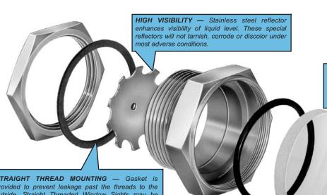
STRAIGHT THREAD MOUNTING — Gasket is provided to prevent leakage past the threads to the outside. Straight Threaded Window Sights may be screwed into tapped holes or used with mounting nuts for drilled holes. Body is constructed of aluminum alloy. Other body material is available on request.
