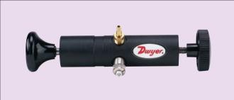
**Serves as pressure source** to calibrate gages and transmitters or to set pressure switches. Use with manometer or other pressure standard. Includes volume adjuster enabling fine pressure control and bleed valve. Generates pressures from a fraction of an in w.c. to 72 psig (5 bar). Includes barbed fitting, tee connector and three 36<sup>°</sup> lengths of vinyl tubing.
