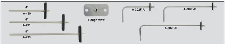
The Stainless Steel Static Pressure Tips are used to measure static pressures in ducts or rooms. They are to be connected to differential pressure switches and transmitters. Two static sensors are used in applications where differential pressure is required across a filter or coil. These sensors include a mounting flange with integral rubber gasket and two screws for simplifying mounting on a duct.
