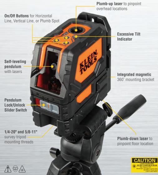
Plumb Spot Laser Horizontal and Vertical Laser Cat. No. UPC 0-92644-Description **Dimensions** Self-Leveling Green 2.6" x 5.3" x 5.0" 93LCLG 93004-1 Cross-Line Laser Level Green Red (66 x 13.5 x 12.7 cm) with Red Plumb Spot Self-Leveling Cross-Line 2.6" x 5.3" x 5.0" 93LCLS 93002-7 Red Red Laser Level with Plumb Spot (66 x 13.5 x 12.7 cm)
