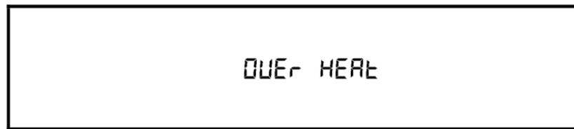
Figure 16 - Over Temperature Protection Warning
