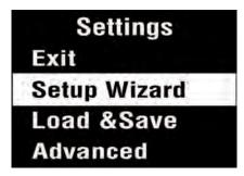
Moving up and down the menu is achieved by pressing the left (up) and right (down) buttons which causes the menu item to be highlighted. Pressing the square button will select the highlighted menu item.
