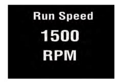
Higher run speeds may need increased BDU threshold values to identify worn or bad bearings. Lower run speeds may need decreased BDU threshold values to identify worn or bad bearings.
