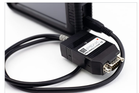
CAN Connections are made by connecting CAN converter to USB port. Diagnostic cable is then plugged into the 9-pin DIN connector and plugged into the vehicle.
