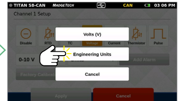
Select Engineering Units
