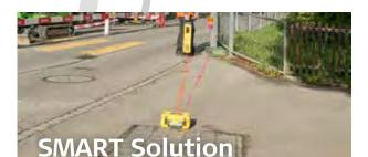
With on board locate alerts and an automatic locate process, the DD SMART locators help to reduce time spen locating buried utilities and prevent utility damage.
