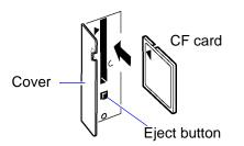
**NOTE** Format a CF card on a computer the first time you use it or before you begin measurement. If the CF card has been used for another purpose, saving may take a while or the file information may be damaged. Formatting will prevent these problems from occurring.
