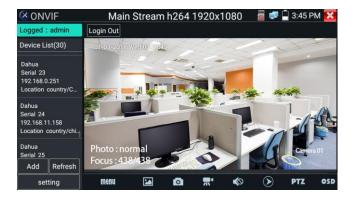
Click the button "Refresh", the tester will scan the ONVIF camera again. Click the newly displayed ONVIF camera on the "Device List". The tester will show the IP camera's relative information and settings.
