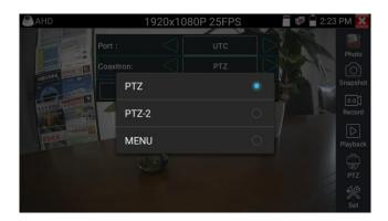
To use coaxial PTZ control with the AHD camera, no parameter settings are needed.
