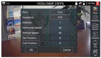
The PTZ address in the tester must be consistent with the dome camera or decoder for the IPC tester to work. After setting the parameter, the tester can control the PTZ and lens.
