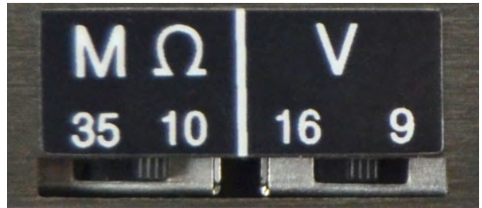
Figure 2. Operator test limit and test voltage switches located on the right-side of the 724 Workstation Monitor
