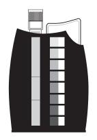
The Octa-Slide 2 Viewer should be held so non-direct light enters through the back of the Viewer. Insert the reacted sample into the top of the Viewer. Slide the Octa-Slide 2 Bar into the Viewer and match the color of the reaction to the color standards.
