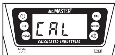
3. Place the level on a flat and smooth surface. Hold the level still for 10 seconds until the display digits stop changing, then press the CAL button, "CAL1" appears briefly in the display.
