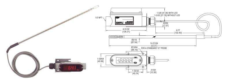
**The Series 641RM** Air Velocity Transmitter uses a heated mass flow sensor technology. It has 8 user selectable ranges from 250 FPM to 15000 FPM with corresponding metric ranges of 1.25 MPS to 75 MPS. The Series 641RM Air Velocity Transmitter provides an isolated 4-20 mA output proportional to the velocity. With the optional 1/2″ 4-1/2 digit LED display, the Series 641RM Air Velocity Transmitter will provide a highly visible local readout of the velocity.
