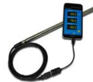
Temperature/ Humidity Sensors
