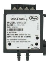
The Series 616KD One-Touch® Differential Pressure Transmitter senses the pressure of air and compatible gases and sends a standard 4 to 20 mA or optional voltage output signal. A wide range of models are available factory calibrated to specific ranges. A single push button properly adjusts both zero and span. New enclosure enables the 616KD to be mounted on a 35 mm DIN rail either via its side or back DIN rail clips.
