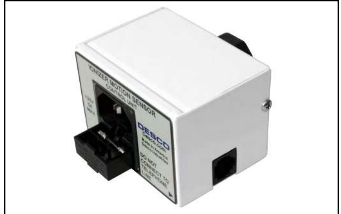
Figure 6. Replacing the fuse in the Control Unit
