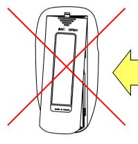
To put the battery cover back, do not first engage the detent at the top end.
