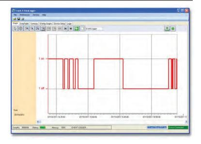
Software automatically calculates total time on, time off, and total test time. Valuable information about run time and power cycling is easily interpreted.
