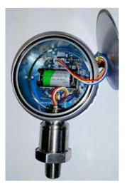
The unit operates off a 1/2 AA 3.6V Lithium battery. The battery is accessed by removing the rear bezel ring and cover. Gently extract the battery and replace as needed. NOTE POLARITY WHEN REPLACING – the unit will not operate if the battery is reversed. Ensure the O-ring is in place before replacing the cover and bezel. Do not stress any of the internal wiring.
