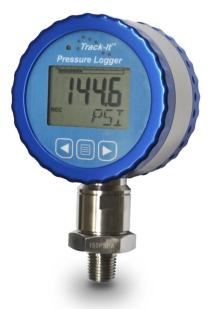
Track-It Pressure/Temp and Vacuum/Temp Data Loggers are packaged in a rugged watertight anodized aluminum and stainless steel housing and have a standard 1/4" NPT fitting. The replaceable internal lithium battery has up to a 3 year life.
