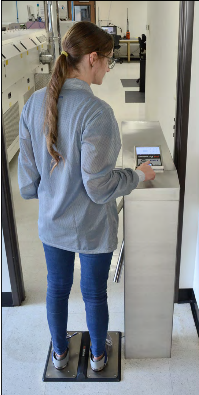
Figure 6. Performing a footwear test
