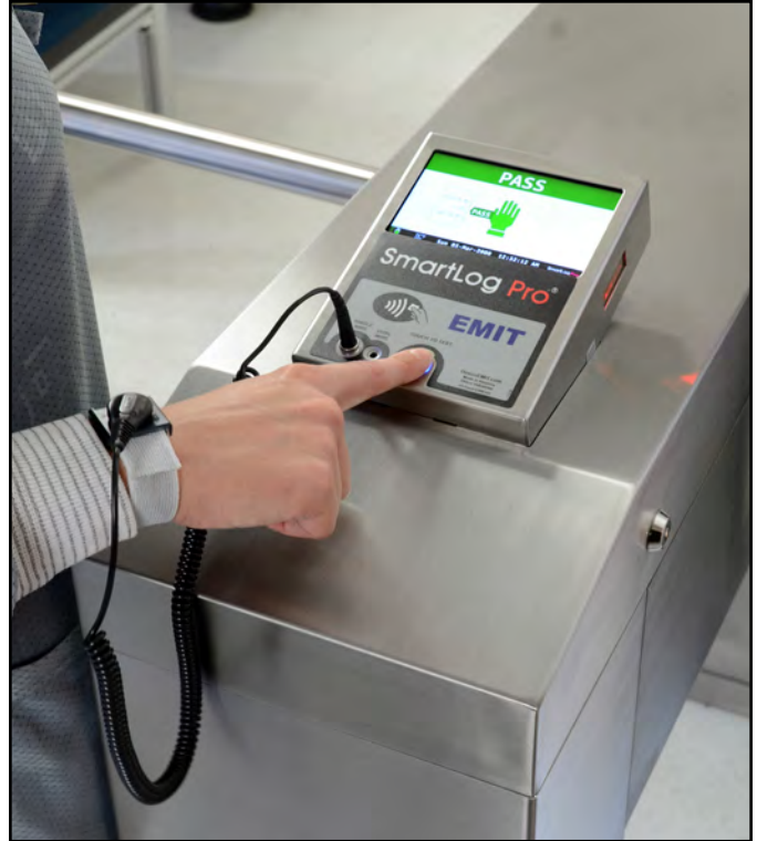
Figure 7. Performing a single-wire wrist strap test
