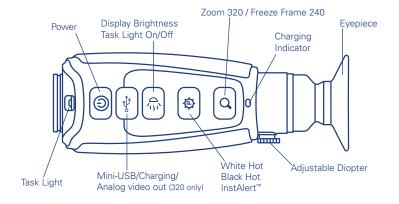
Power Button – Ocean Scout<sup>™</sup> has three power states: On, Off, & Auto Shutdown. • On – Takes approximately 4 seconds (during bootup the FLIR splash screen
