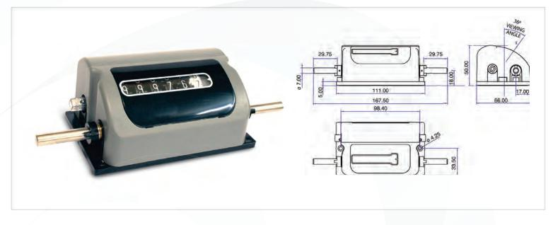
This unit counts revolutions on many different types of production machinery. Robustly constructed for continuous operation at high speeds with the main shaft running in double oil impregnated bearings to ensure accurate, long term, trouble free service. It is supplied with a double drive with wing bush, customer configurable reset.
