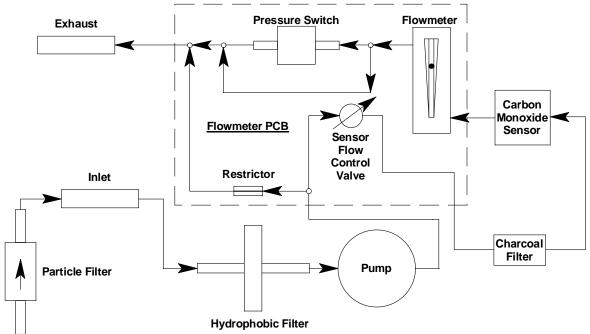
Figure 2: Carbon Monoxide Sample-Draw Detector Flow Diagram
