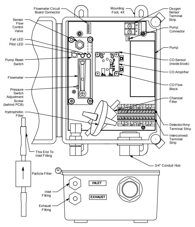
Figure 1: Carbon Monoxide Sample-Draw Detector Component Location
