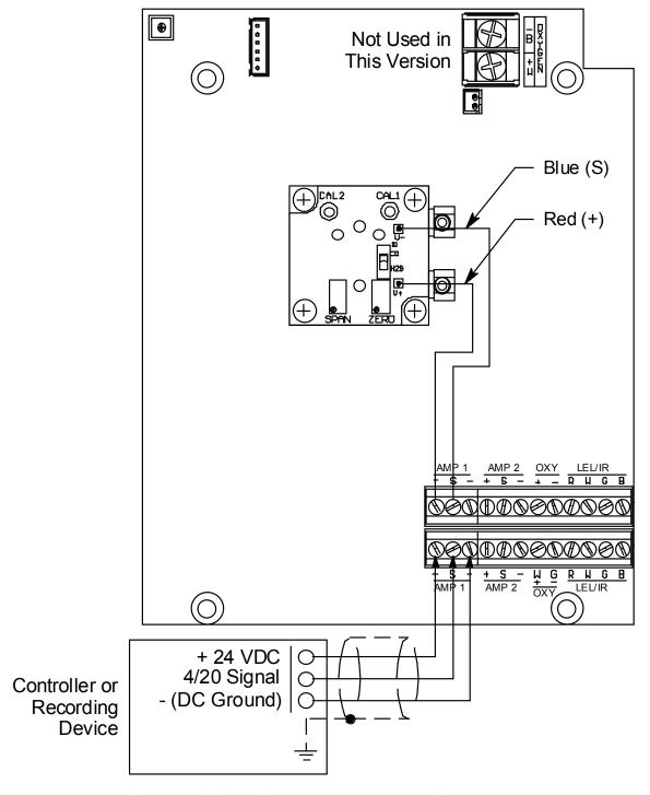
Figure 5: Wiring the Sample-Draw Detector to a Controller
