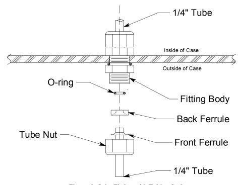
Figure 6: Inlet Fitting with Tubing Stub
