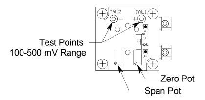
Figure 3: CO Amplifier Component Location
