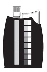
The Octa-Slide 2 Viewer should be held so non-direct light enters through the back of the Viewer. Insert the reacted sample into the top of the Viewer. Slide the Octa-Slide 2 Bar into the Viewer and match the color of the reaction to the color standards.
