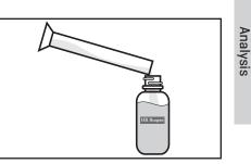
2. Use the 5 mL volumetric pipet (0329) and pipette pump (30527) to add 5 mL of Indigo Blue Stock Solution (3989) to the amber glass bottle. Cap and mix.
