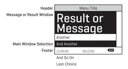
As described previously, the EXIT button allows an exit or escape from the current menu and a return to the previous menu. This allows a rapid exit from an inner menu to the main menu by repeatedly pushing the EXIT button.
