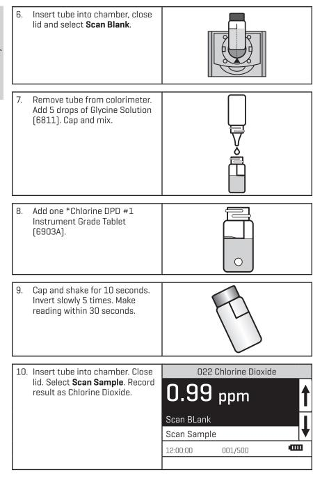
NOTE: The meter will remember the last scanned blank reading. It is not necessary to scan a blank each time the test is performed. To use the previous blank reading, instead of scanning a new one, scroll to Scan Sample and proceed. For the most accurate results, the meter should be blanked
