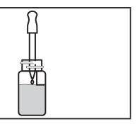
10. Use the 1.0 mL pipet (0354) to add 2 measures of \*Acid-Zirconyl SPADNS Reagent (3875). Cap and mix thoroughly. (This is the reagent blank.) Dry the tube with a lint-free cloth.
