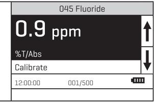
13. Press enter to select **Calibrate**. A reverse font (light background with dark characters) will appear to indicate that the reading can be adjusted.
