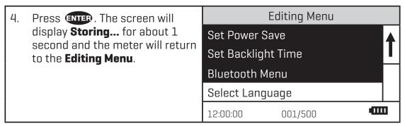
NOTE: If meter unintentionally switches to another language, use the procedure above to reset the meter to the desired language. For example, to reset the meter to English:
