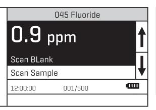
NOTE: Zeroing the meter with the sample water will result in an error. Meter must be zeroed with a reagent blank.
