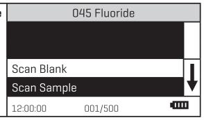
5. This test requires a reagent blank. Rinse a clean colorimeter tube (0290) with clear, colorless, Fluoride free water. Fill to the 10 mL line with clear, colorless, Fluoride free water.
