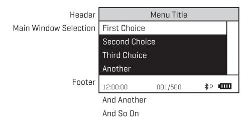
A light bar will indicate the menu choice. As the menu is scrolled through, the light bar will highlight different menu choices. Pressing the select the menu choice that is indicated by the light bar.
