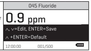
14. Press or to adjust the value shown to the concentration of the prepared standard, 1.0 in this example.
