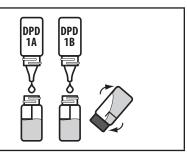
Immediately insert tube into chamber. Close lid. Select **Scan Sample**. Record result as Free Chlorine.
