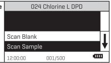
Rinse a clean tube (0290) with sample water. Fill to the 10 mL line with sample. Cap and wipe dry.
