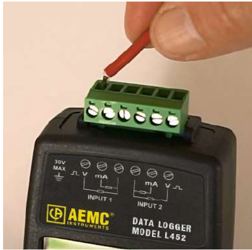
Figure 24. Inserting a lead into the terminal strip
