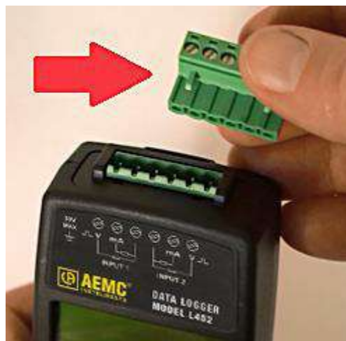
Figure 23. Terminal strip (upper right)
