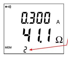
The measurement is recorded in the memory slot of which the number is displayed (in this example, slot number 2).
