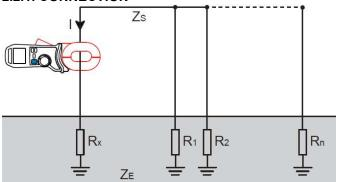
The ground electrode to be measured (R<sub>X</sub>) is in a series/parallel arrangement with other ground electrodes via the earth impedance (Z<sub>E</sub>) and physical connection to other resistance paths (Z<sub>S</sub>). The measured impedance will be slightly greater than R<sub>X</sub> assuming the downstream impedance is very low. For example: If R<sub>X</sub> is 21 $\Omega$  and Z<sub>S</sub>/R<sub>1</sub>-R<sub>n</sub> is effectively 0.6 $\Omega$ , the Model 6418 will read 21.6 $\Omega$ .
