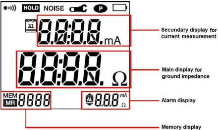
When the measurement exceeds the limits of the measurement range, the instrument displays **OR**.
