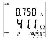
If you set alarms on both the impedance and the current, and both alarm thresholds are exceeded, the alarm on the current has priority.
