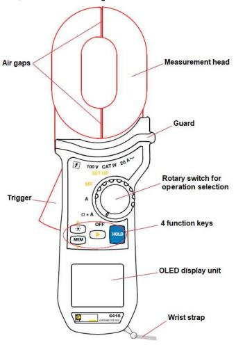
Clamp-On Ground Tester Model 6418
