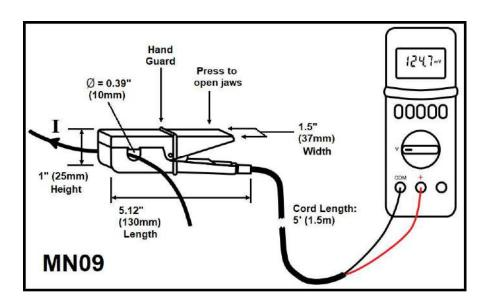
Output Signal: 100mV = 1A<sub>AC</sub>
