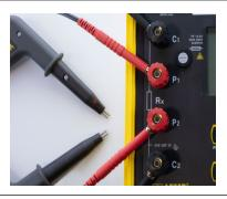
\*For Models 6240 and 6255 instruments with serial numbers lower than 1166339SEDV, terminals C1 and P1 are red, and C2 and P2 are black. In this case, connect probes as shown in the table on the following page.
